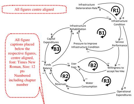
Figure 1.1: Feedback loops in water and wastewater network management.
