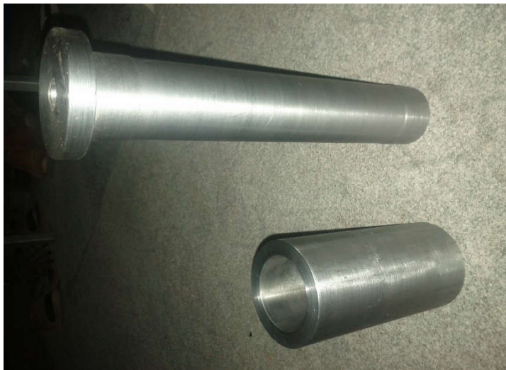
Figure 5: Die for formation of blocks
