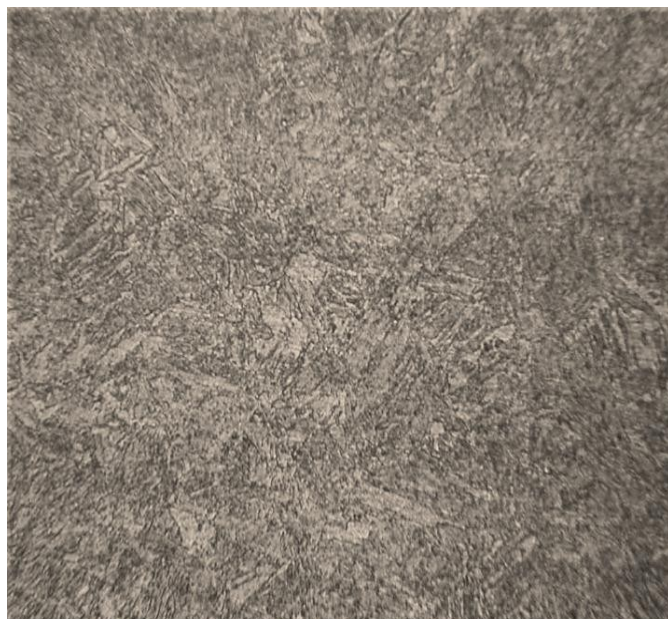
Figure 6 Microstructure of tubing cross section (Magnification x800)
