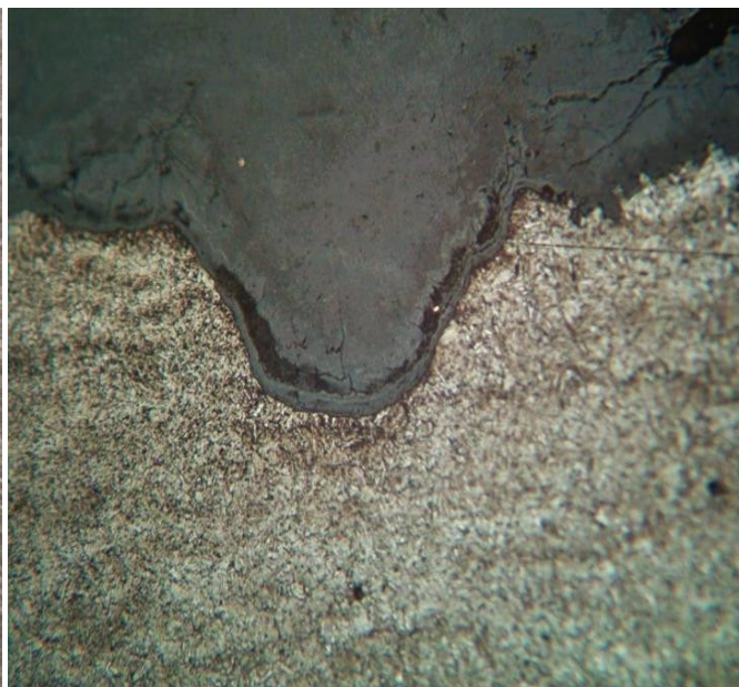
Figure 7 Microscopic images showing small pits in the tubing cross section (Magnification x200)
