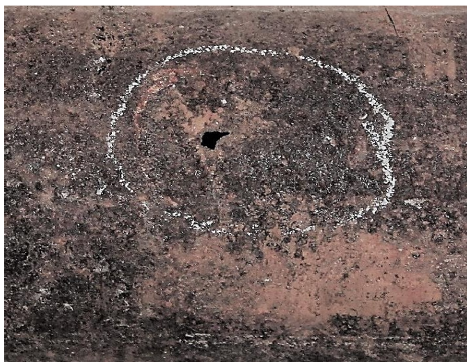
Figure 2 Puncture observed from outside of tubing
