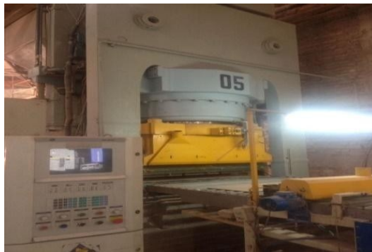
Fig.4: Press Machine presses the powder into the desired size
