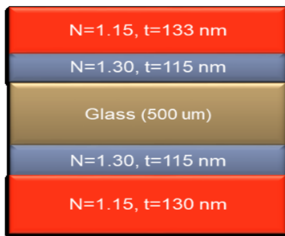
Fig.2 Thin film stack of silica nanoparticles on Glass substrate on both side modelled through MRT software
