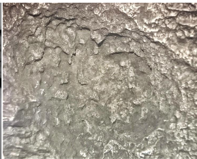
Figure 5 Inner surface of tubing after cleaning of corrosion products and deposits
