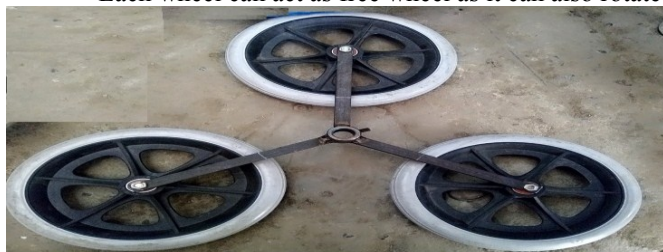
Figure2. Tri-wheel mechanism for automatic stair climbing wheelchair.
