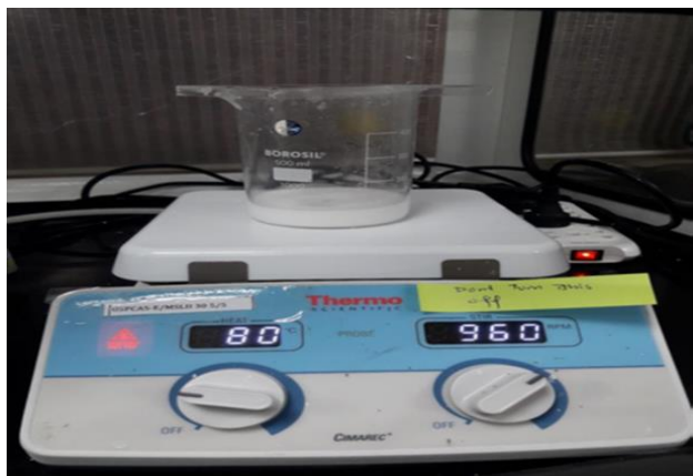
Fig. 2. Experimental setup of preparing 30 Vol% starch solution, hot plate is used with magnetic stirrer, the temperature was kept constant at 80 °C while mixing speed was 960 rpm for 24 hours.
