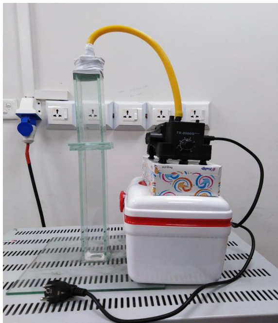
Fig. 10. Visual Permeability Test Setup, All the dimensions of the glass tube is according to the dimensions of the prepared membrane samples. The height of the lower glass tube is 10 inch while the upper glass tube part have 6 inch in length.
