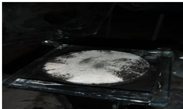
Fig. 10. Visual Permeability Test Setup, All the dimensions of the glass tube is according to the dimensions of the prepared membrane samples. The height of the lower glass tube is 10 inch while the upper glass tube part have 6 inch in length.
