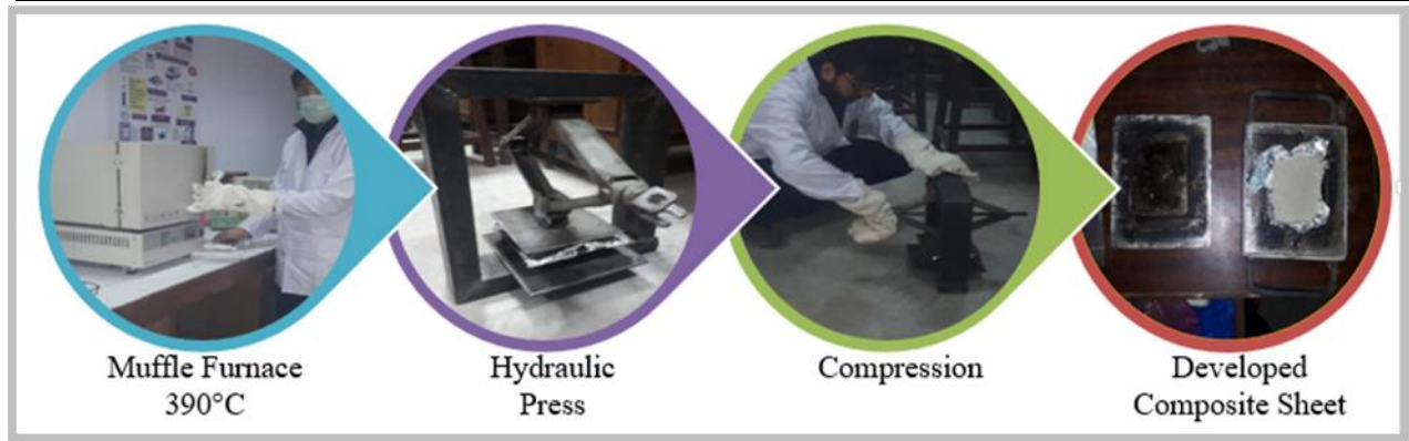
Fig 2. Schematic of fabrication of composite sheet
