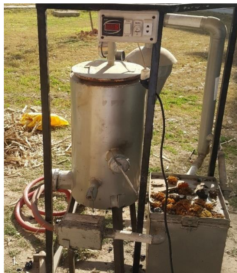
A. Creo model of downdraft biomass gasification system B. Fabricated downdraft biomass gasification system
