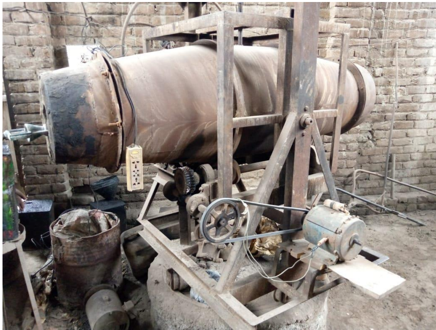
Figure 2 Rod mill for sample preparation and finish grinding at Department of Mining Engineering, UET Peshawar
