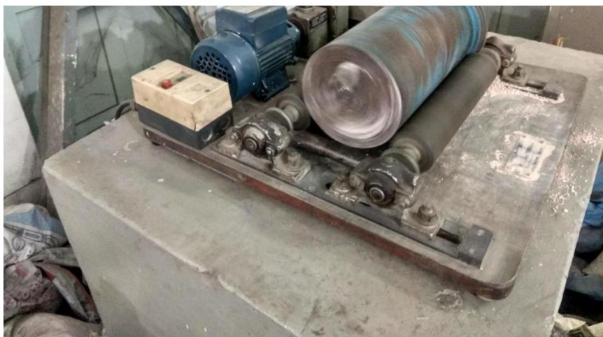
Figure 3 Lab scale rotary kiln utilized for the production of cement clinker.
