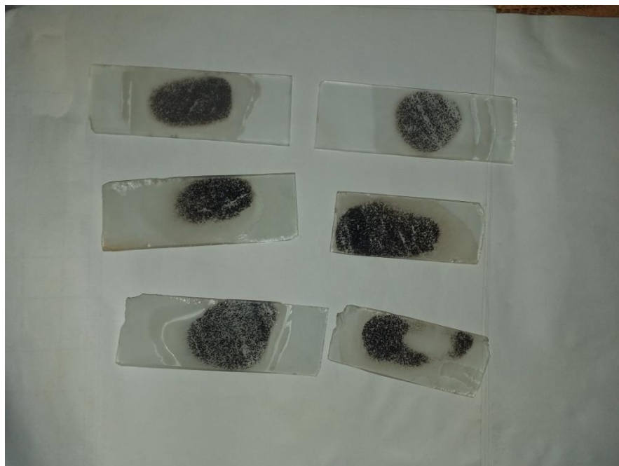
Fig. 1. Six representative thin sections of Kohistan chromite ore.
