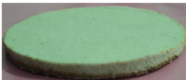
Fig. 4. Front side view of sample-01 (50 wt% alumina and 50 wt% fly ash) membrane sintered at 1250 °C
