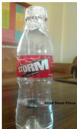
Fig. 1. Mild steel piece in solution for Weight Loss method
