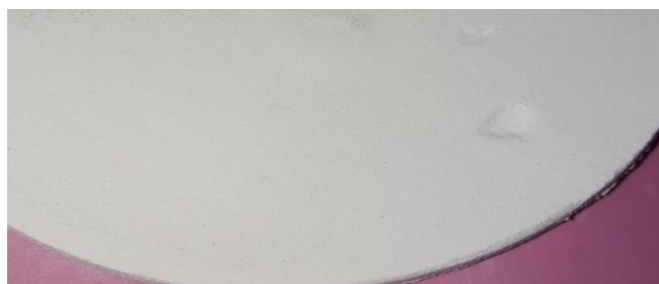
Fig. 5. Top side view of sample-04 (66.3 wt% alumina and 33.3 wt% fly ash) membrane sintered at 1250 °C
