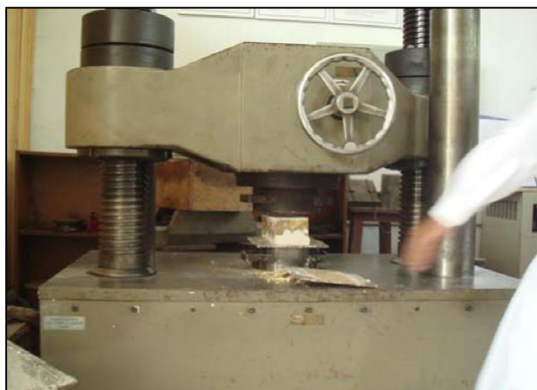
Figure 5. SCEB Compression test in Universal Testing Machine
