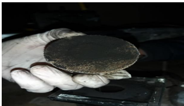
Fig. 11. Cake of blackish particulates over the lower surface of membrane exposed to flue gases from
