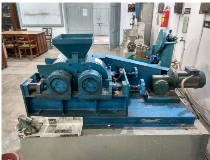
Figure 1 Double roller crusher for sample crushing at Department of Mining engineering
