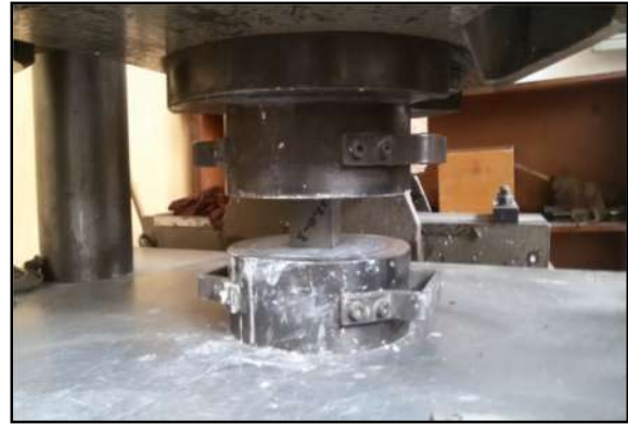
Figure 1: Compressive Strength Test of mortar Cube in UTM
