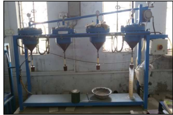
Figure 3: Permeability Test Apparatus
