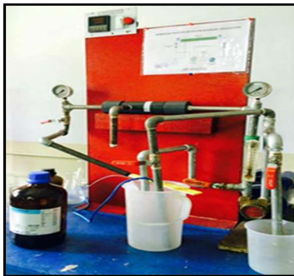
Figure 2A: Experimental Setup of Lab scale Membrane Reactor
