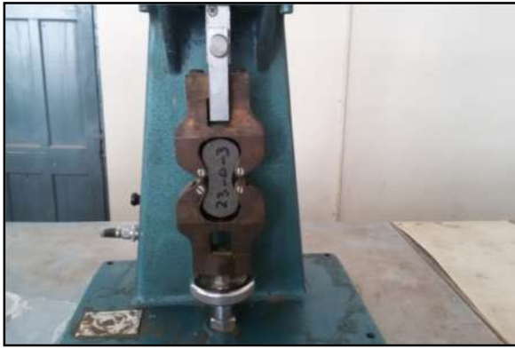
Figure 2: Tensile Strength Test of Briquette
