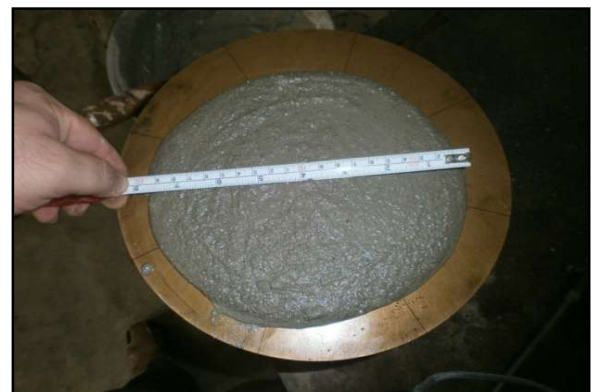
Figure 4: Flow of Mortar Specimen on Base of Flow Table
