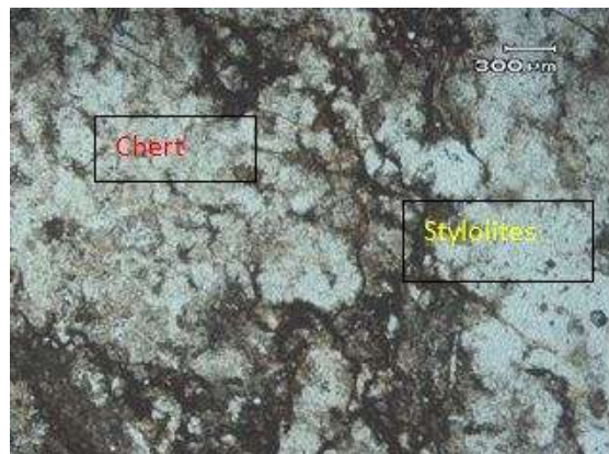
Figure 1. Chert embedded in dolomitized lime mud matrix.
