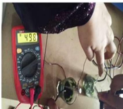
Figure 3: Bio E-Cell in Cascade Setup
