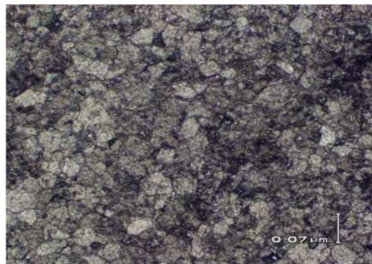
Figure 4: Photomicrograph of cryptocrystalline Micritic calcite grains.
